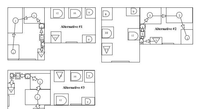
Figure 4 The alternative facility layout for germinate brown rice mill.
